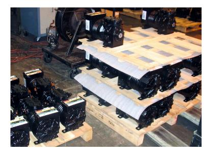
The fully packed skid is shrink wrapped, and a "box" label is applied over the wrap. At this point, a final verification is made of all contents on the skid. Operators scan the license plate, model, customer order, sequence, and customer part number information from the skid and compressor labels. If all scanned information matches with the database, then that skid is released to shipping. However, if something is amiss, the system once again alerts the operator that there is a problem.
