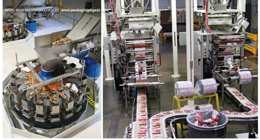
Two radial weighing systems, above left, feature 18 individual weigh heads each to keep up with the speed of the vertical form/fill/seal machines, above right. Jelly Belly beans discharge through metal detectors installed between the scales and the bag machines and continue into the bags being produced below.
