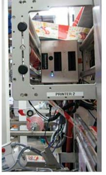
Two thermal-transfer printers print selected information on the film as it travels up the back of the vertical form/ fill/seal machine, above. Operator stations are mounted next to the machines, below, for easy access.
