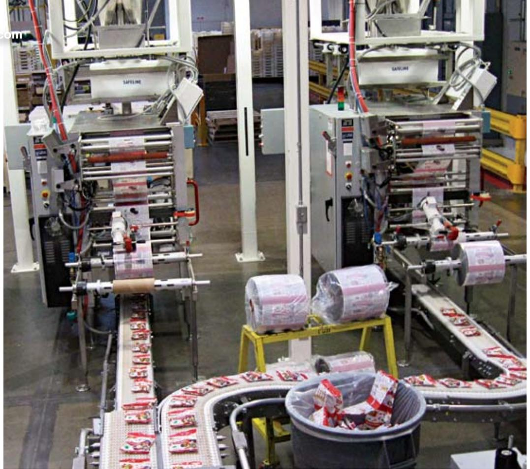
Two radial weighing systems, above left, feature 18 individual weigh heads each to keep up with the speed of the vertical form/fill/seal machines, above right. Jelly Belly beans discharge through metal detectors installed between the scales and the bag machines and continue into the bags being produced below.
