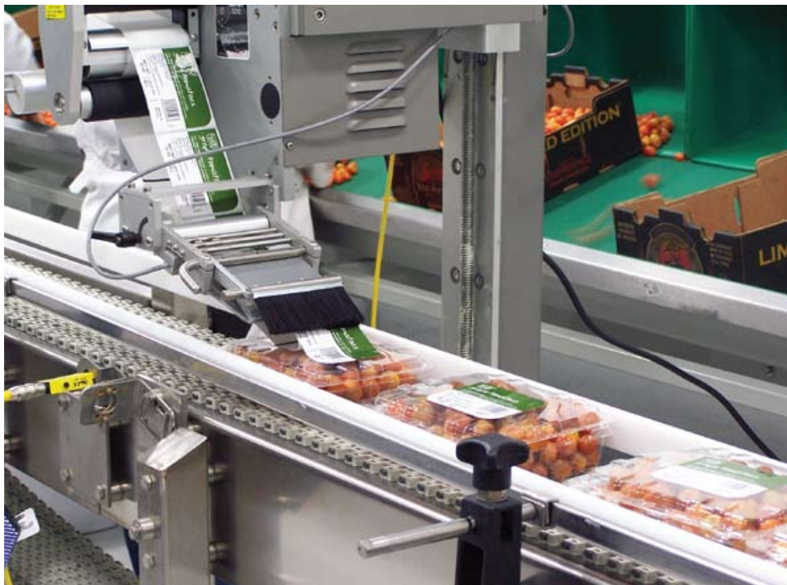
SPEEDIER APPLICATION. Pressure-sensitive labels are applied to the tops of the clamshells at approximately 50/min.
